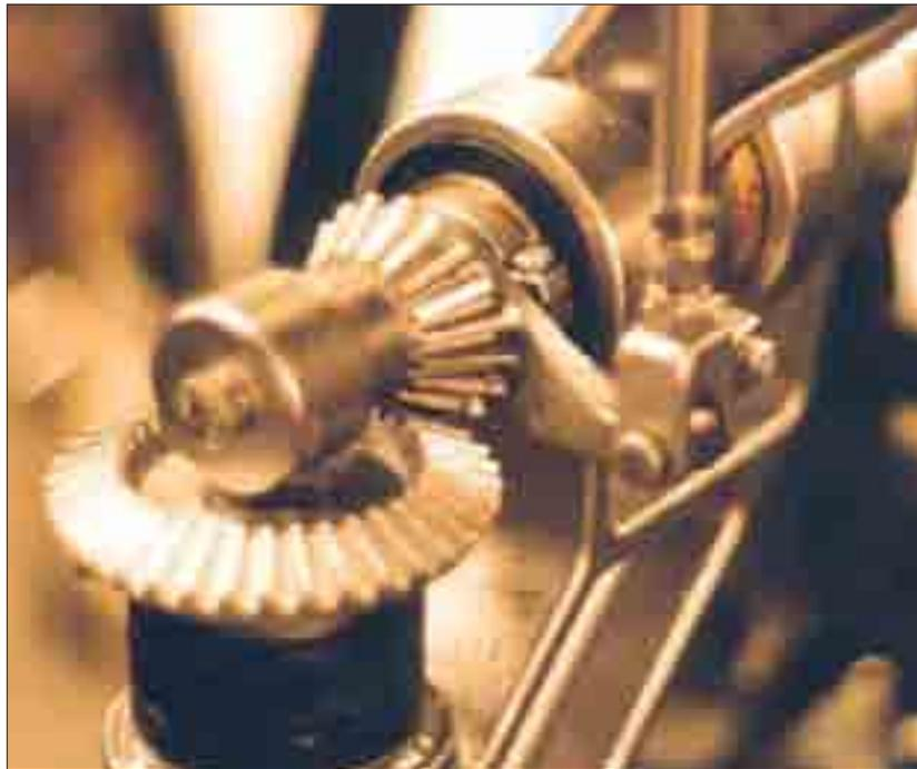
The bevel gear is used to change the axis of rotational motion. By using gears of differing numbers of teeth, the speed of rotation can also be changed.
